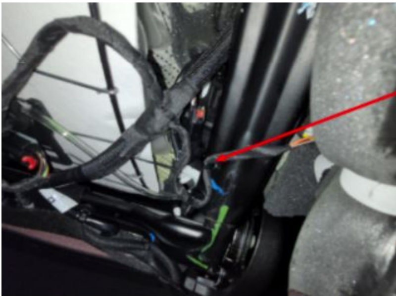
6. Zip tie the airbag connector harness to the seat frame.
