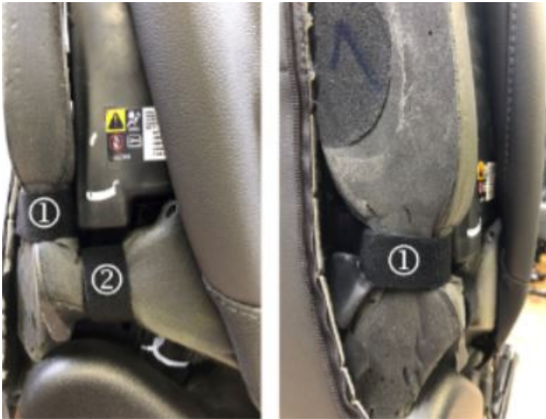
7. Cut 2 pieces of 1" wide double-sided Velcro tape P/N 189590, or equivalent, one 200 mm (7.84 in.) length and the other 180 mm (7.08 in) length.
