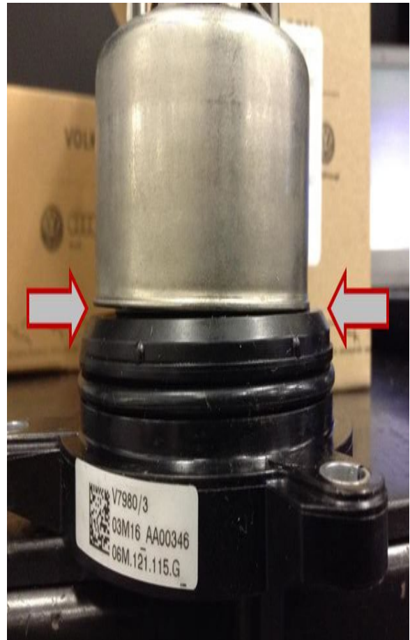
Figure 1. Gap between chamber and seal.
