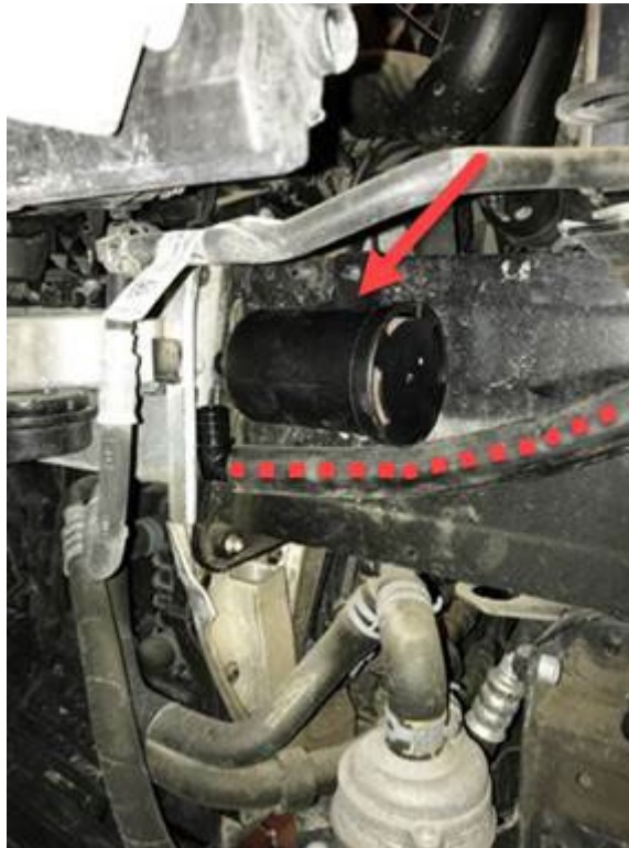
Figure 3. Installing the new NVLD filter.
