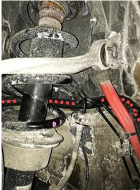
Figure 6. Routing the rubber hose.
