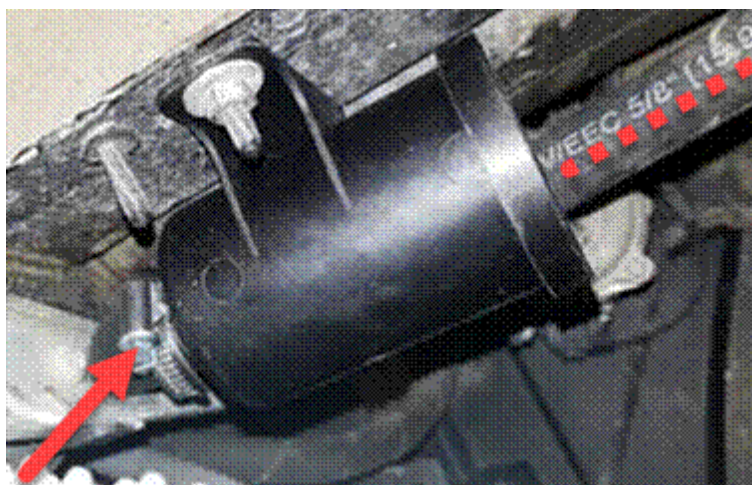
Figure 4. Connecting the NVLD filter.
