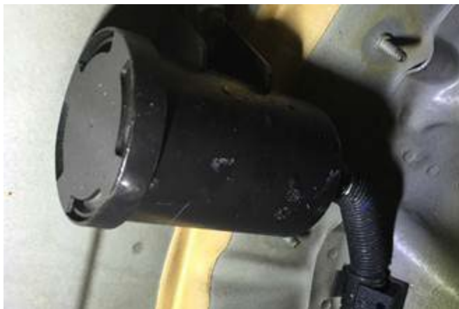
Figure 2. Ventilation tube of the EVAP canister.
