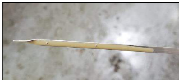
Figure 2. Engine Oil (Milky/Discolored)
