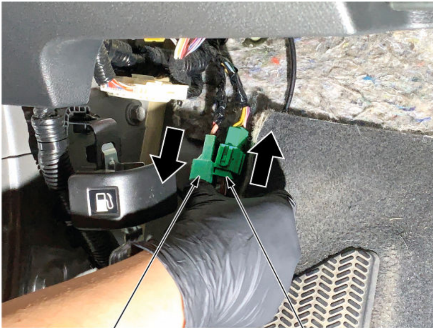
ENGINE ROOM HARNESS CONNECTOR Slide apart.
