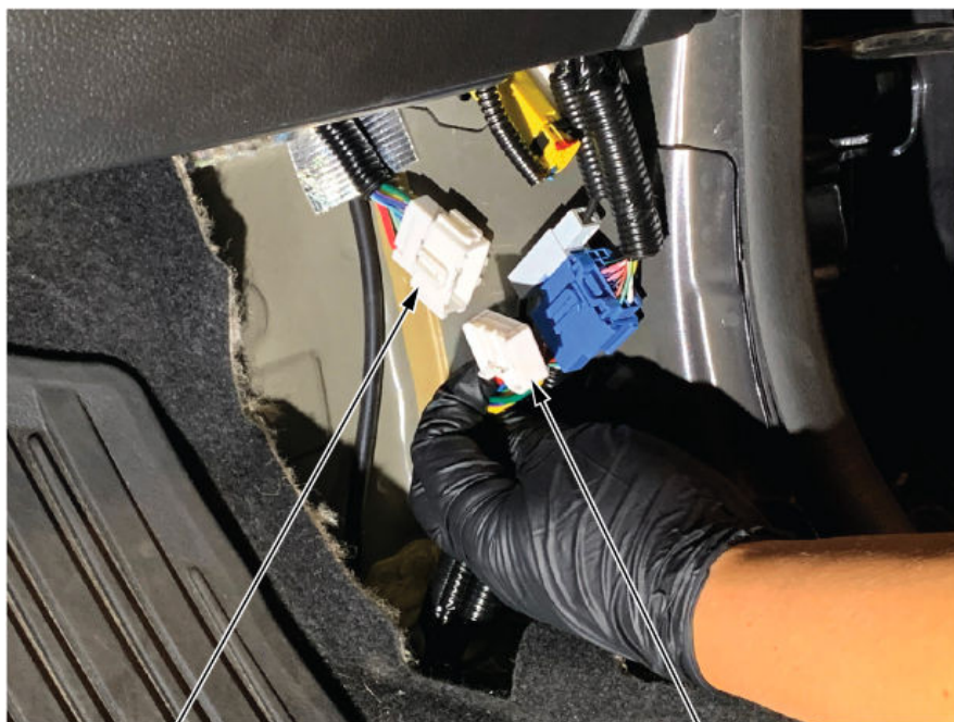
ENGINE ROOM HARNESS CONNECTOR Disconnect.
