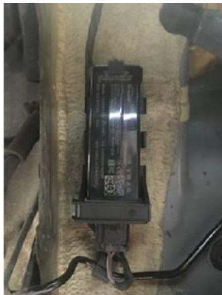
Figure 2. Installation location with new bracket 4E0 810 675 C.
