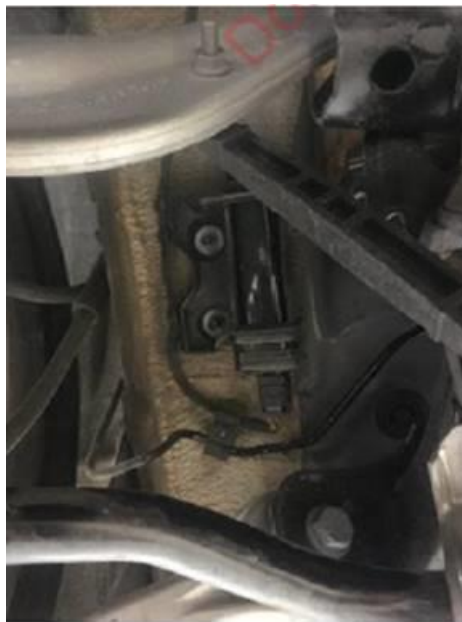
Figure 1. Installation location with standard bracket 4K0 907 249 A.
