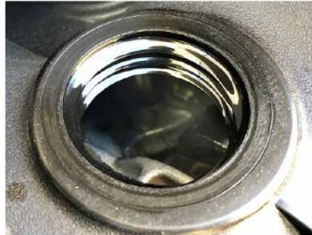
Oil filler opening: Clear view inside opening.
