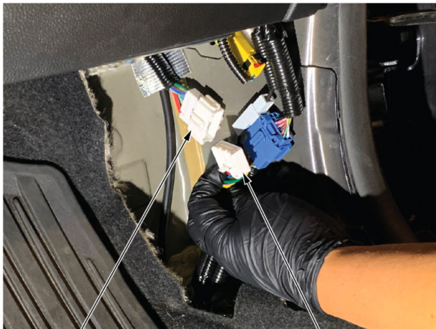
ENGINE ROOM HARNESS CONNECTOR Disconnect.
