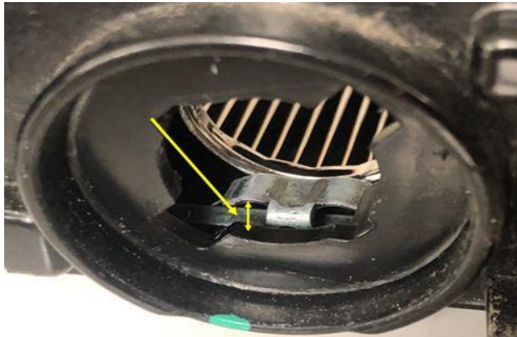
Figure 1. Tail lamp contact loose/pulled away from housing.
