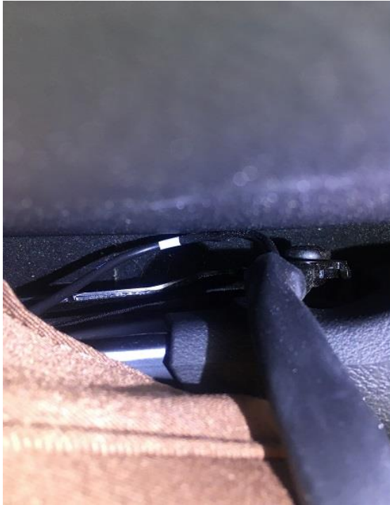
Figure 2. Belt buckle wiring from buckle to seat frame.
