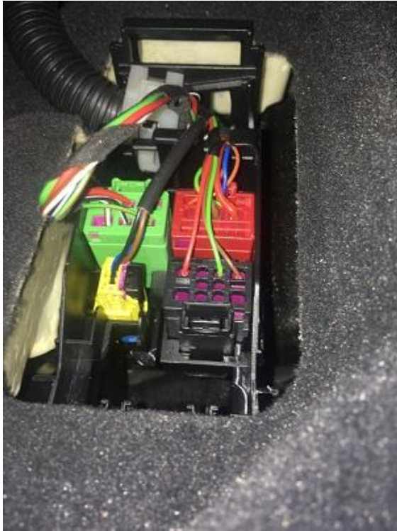
Figure 4. Belt buckle wiring and connector in coupling station.
