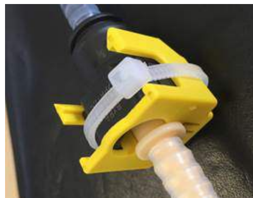
Figure 8. Cable tie installation.
