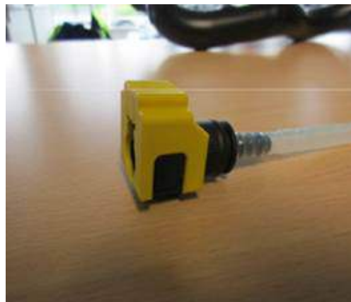
Figure 4. Securing clip correctly installed with the release tabs locked in place.
