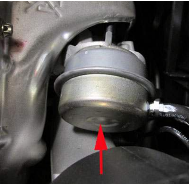
Wastegate Preload Inspection.
