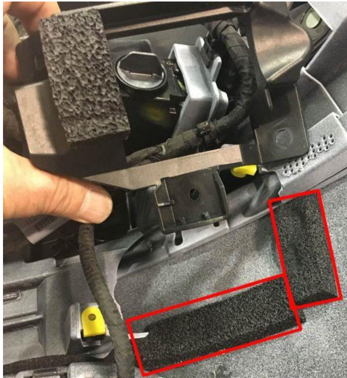
Figure 4. Foam to be stripped out.
