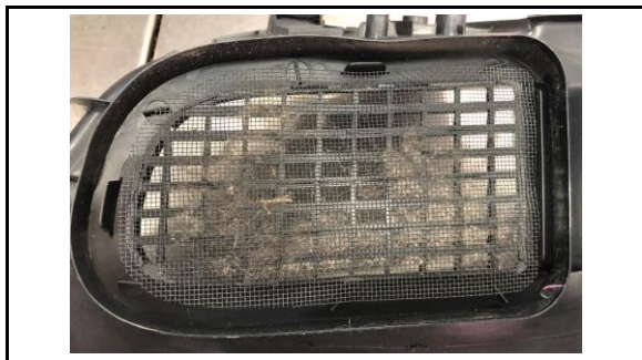
Figure 5. Example of a Dirty RAV4 HV Battery Cooling Intake Filter
