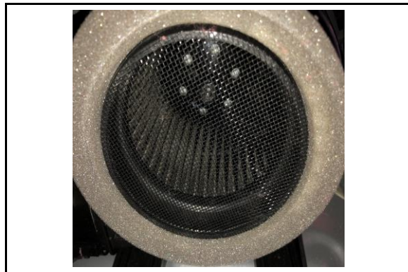
Figure 4. Example of a Clean Prius C HV Battery Cooling Filter
