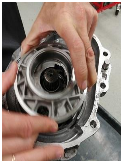
Figure 10. Gear carrier removal.
