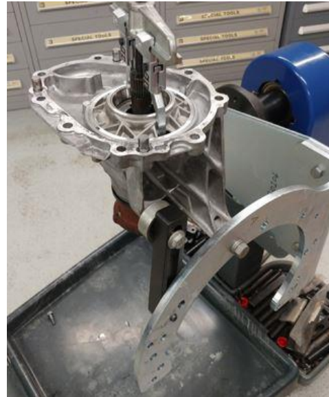
Figure 3. Mounted side carrier.
