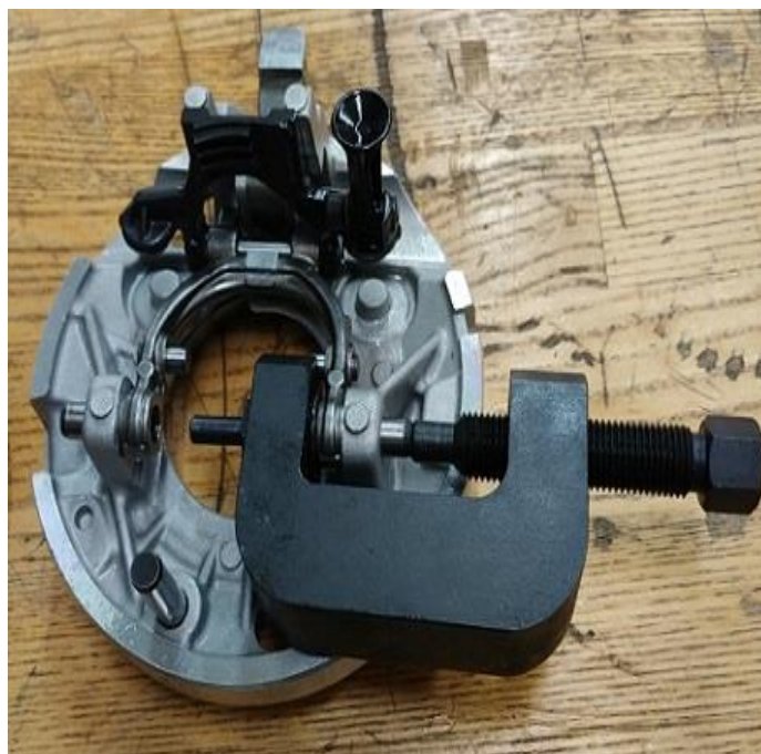
Figure 18. Pin pressing with the 582277.
