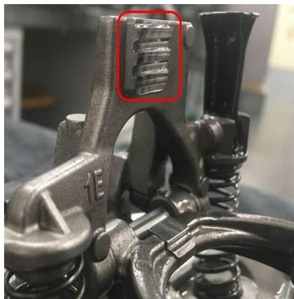
Figure 1. Worn/faulty shift fork.
