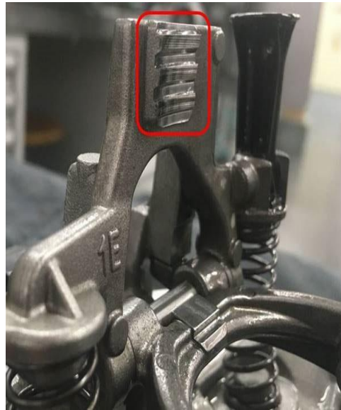
Figure 1. Worn/faulty shift fork.
