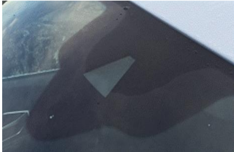
Figure 1. Viewing area fogged up from outside.
