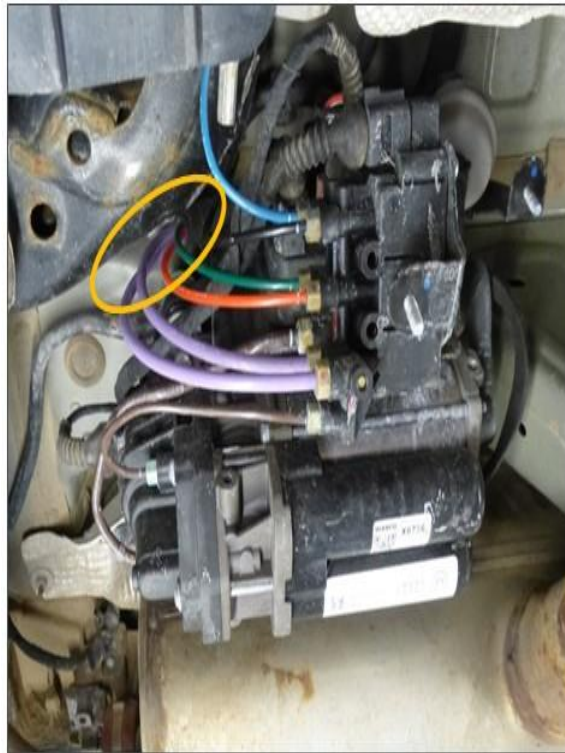
Figure 1. Checking the air hoses.
