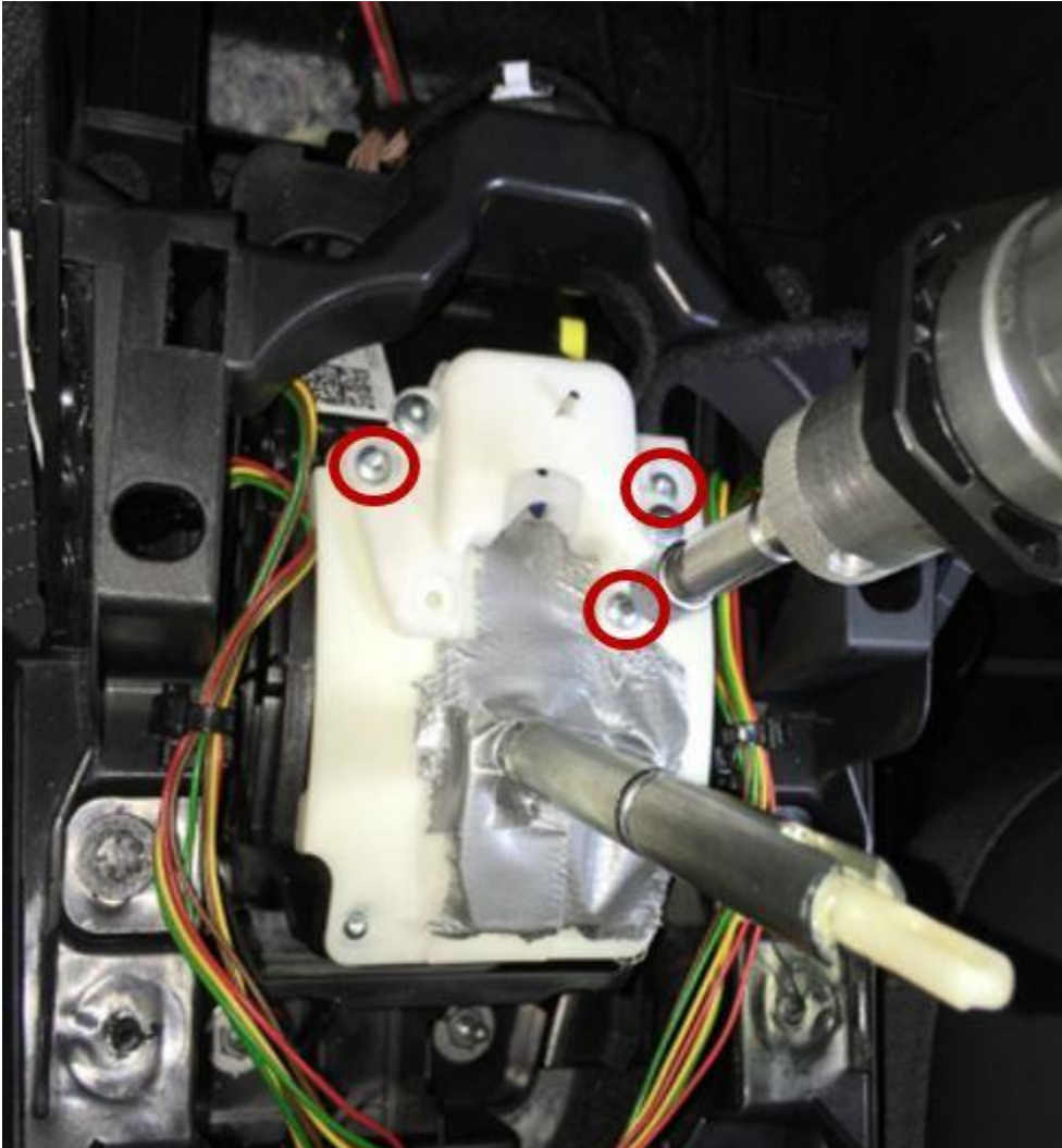
Figure 10. Installing the microswitch module.
