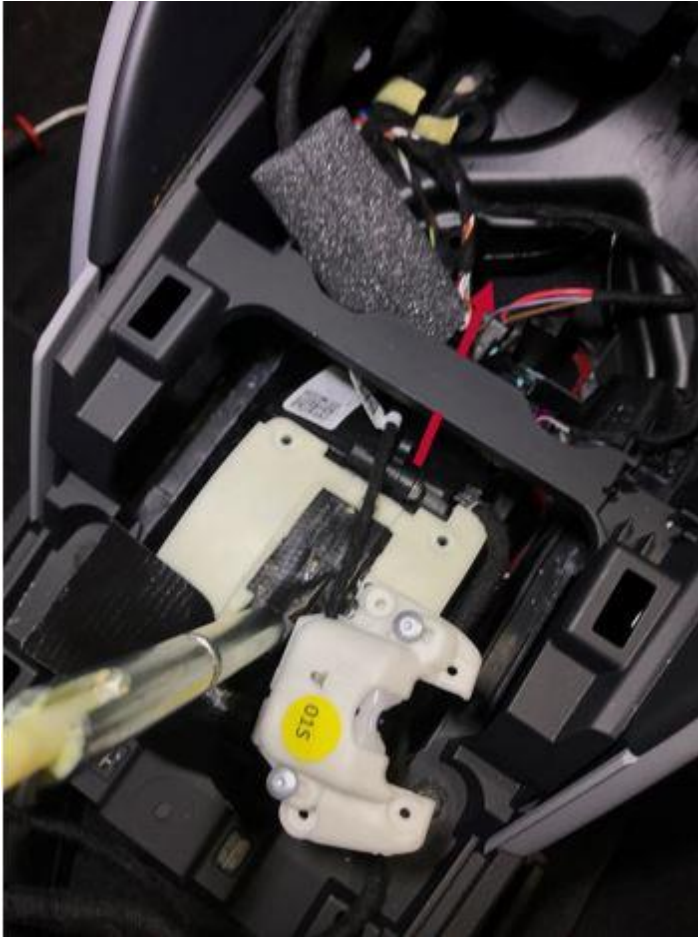
Figure 8. Wiring harness run under the crosspiece.
