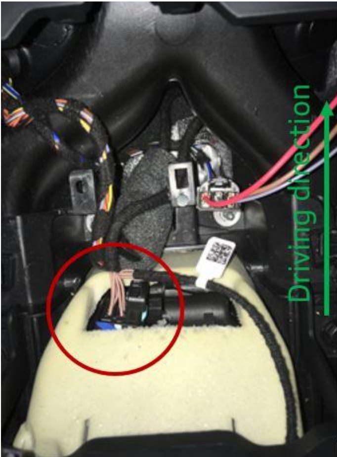
Figure 3. The electrical connection of the selector lever control module.
