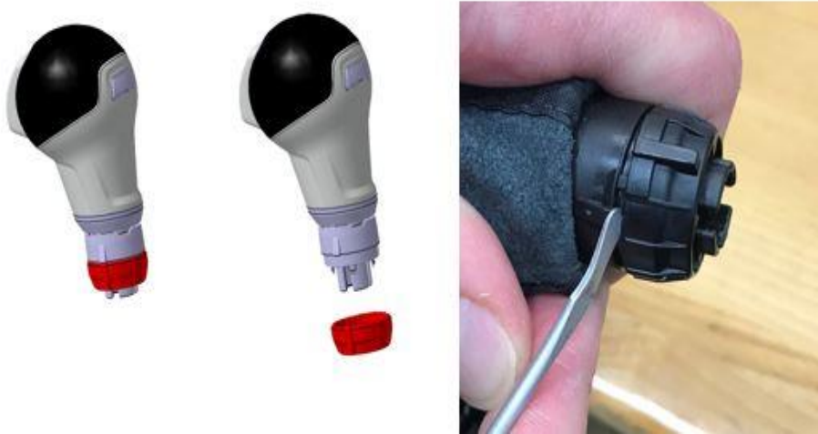
Figure 14. Locking collar removing.
