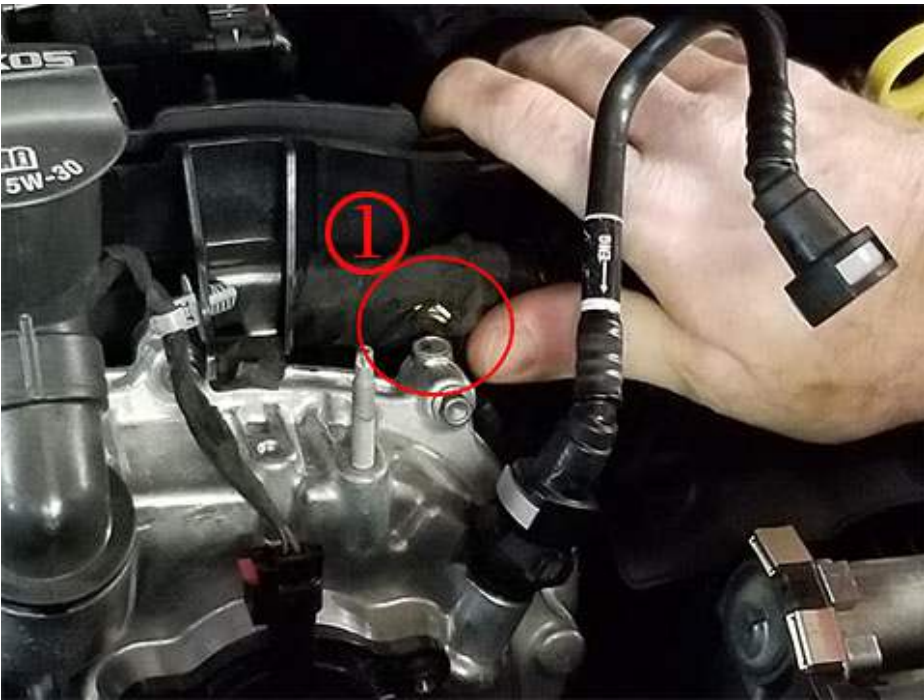
Inspect the engine harness at the Lower Air Cleaner Housing as shown below.
