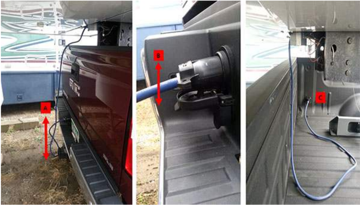
3. Poor trailer wiring connections, as shown below. General Motors does not recommend these type of connections, but many trailers utilize these connections. These type of connections are not robust and are not recommended, especially for brake wiring.
