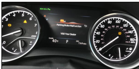
Figure 1. Parking Brake Malfunction Warning Message
