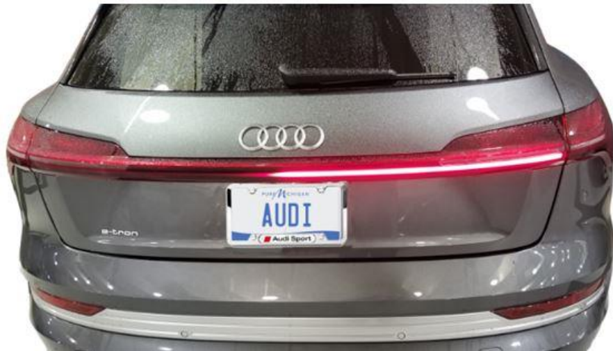
Figure 1. Partially lit trunk lid taillight.
