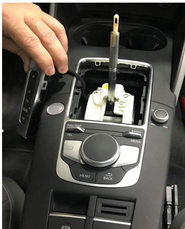
Figure 13. Console insert installed.
