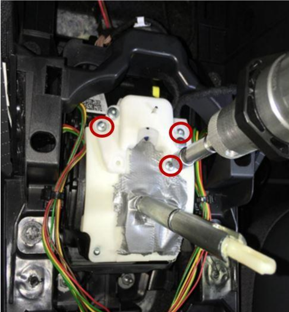
Figure 10. Installing the microswitch module.
