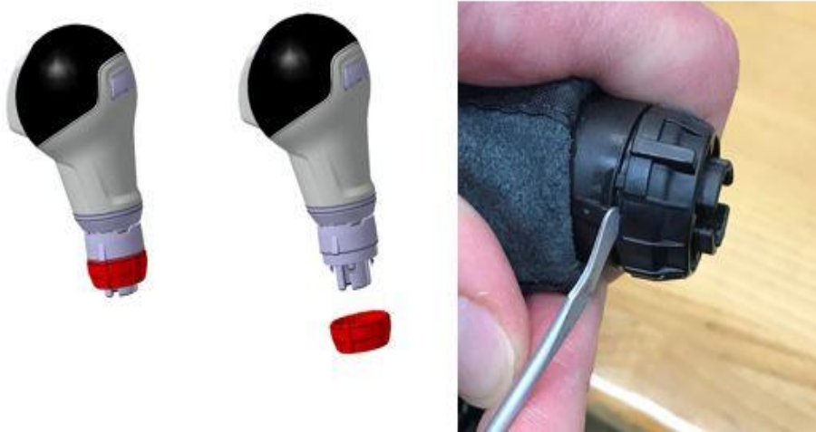
Figure 14. Locking collar removing.
