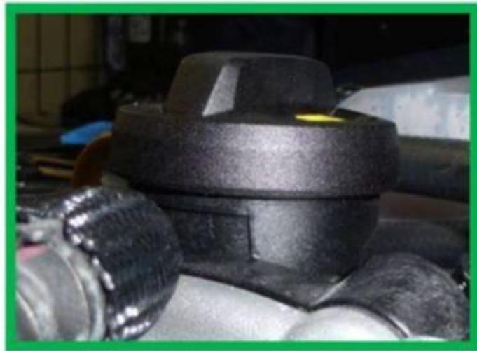
Figure 2. The image bordered in red is an incorrectly installed oil filler cap; a correctly installed oil filler cap is bordered in green.
