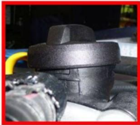
Figure 2. The image bordered in red is an incorrectly installed oil filler cap; a correctly installed oil filler cap is bordered in green.
