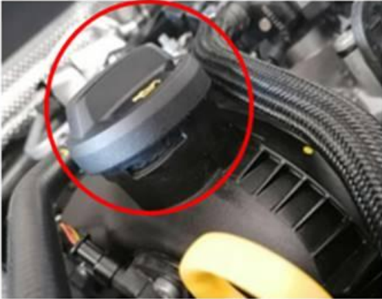
Figure 1. An incorrectly installed oil filler cap.
