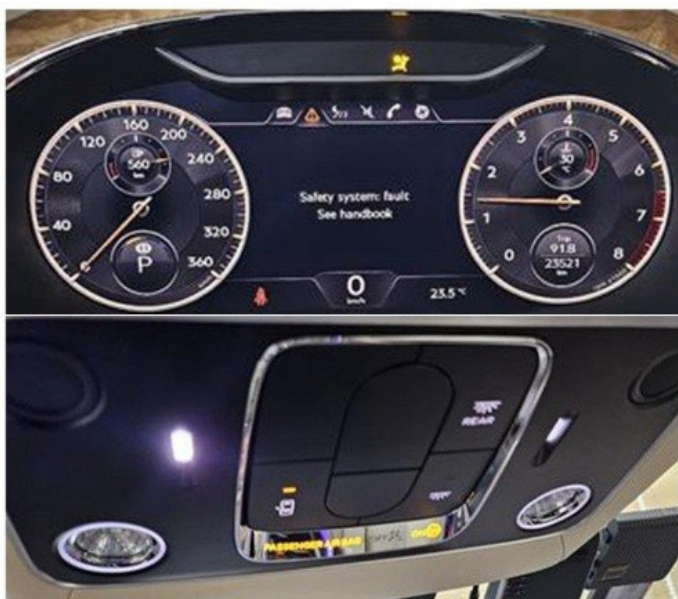
Figure 1. Airbag warning illuminated in the instrument cluster
