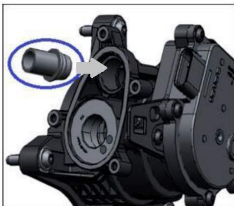
Fig. 1: Shows correct orientation with the flat side (or short end) of the dummy plug (with o-ring) going into the upper hole (see arrow) of the CCV.
