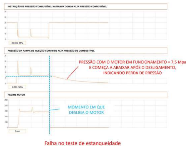
Fig. 2 Leak Test - KO Result
