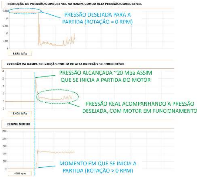
Fig. 2 Engine Start With Failure
