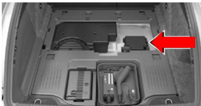
Fig. 2 Rear PDC Location
