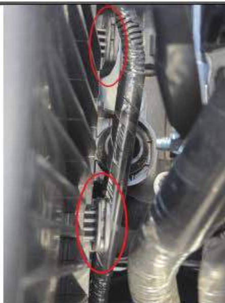
Properly inserted upper and lower tabs. The air box is sealed from the turbulent underhood air.
