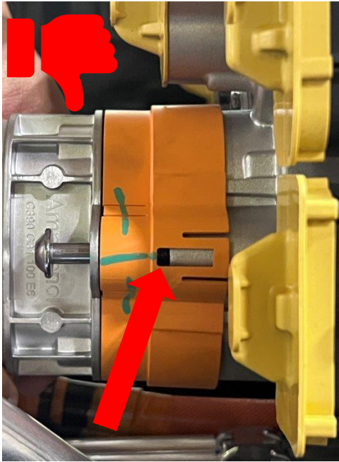
Not Good: Air Gap in Window
