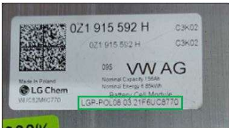
Figure 1. Example image of a battery module type plate with production date: 08 03 21 (= 08.03.2021).
