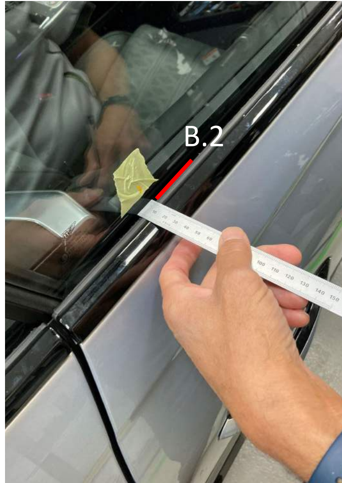
Measure from first lip rubber seal to window glass (B.2)
