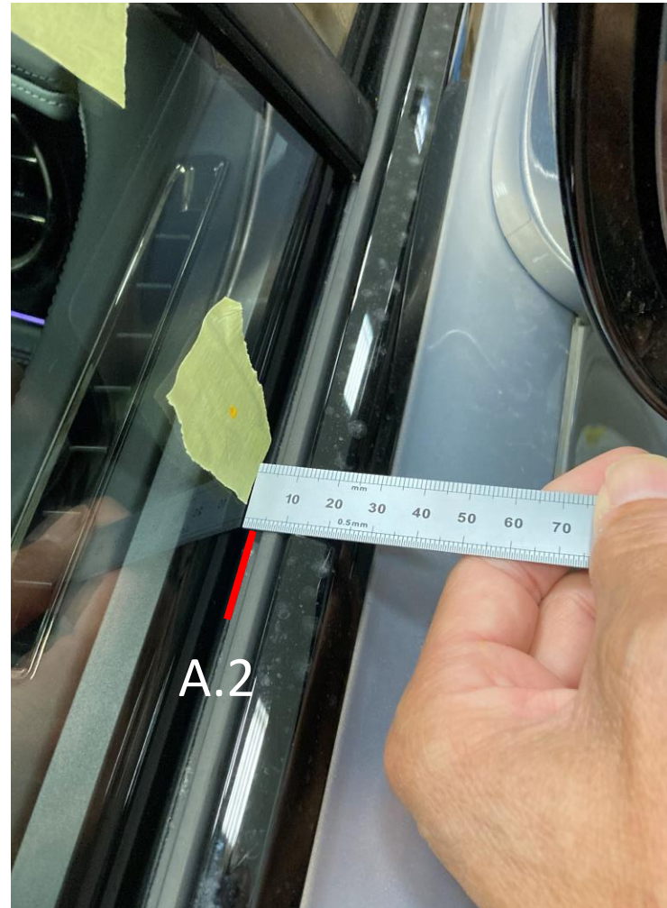
Measure from first lip rubber seal to window glass (A.2)
