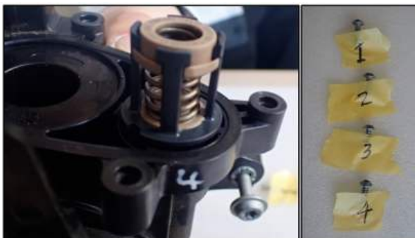
Marking Example 2: Number each screw and their respective hole as shown above.
