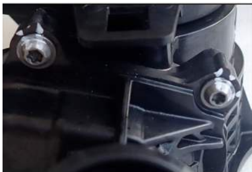
Marking Example 1: Draw marking lines over the screws and the thermostat cover as shown above.
