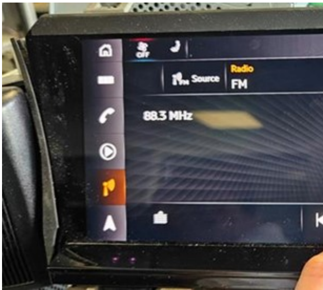
Figure 4. The MIB is in fallback mode if the ambient temperature is not displayed in the upper-left corner of the screen. Please note this will appear on the right hand side on right hand drive vehicles.
