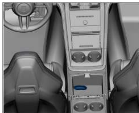
Place remote control in emergency start tray
