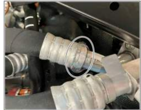
Example of a leak on pressing with alkali/soapy water
