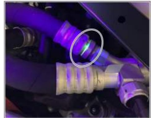
Example of a leak on pressing with leak detection additive
