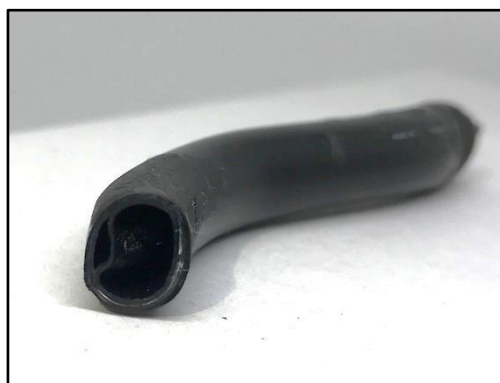
Restricted Fuel Line
