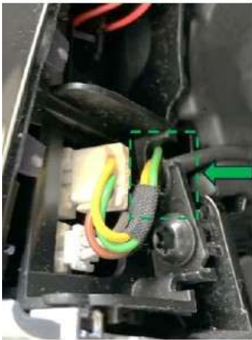
Figure 2. Correct wire routing on left side.
