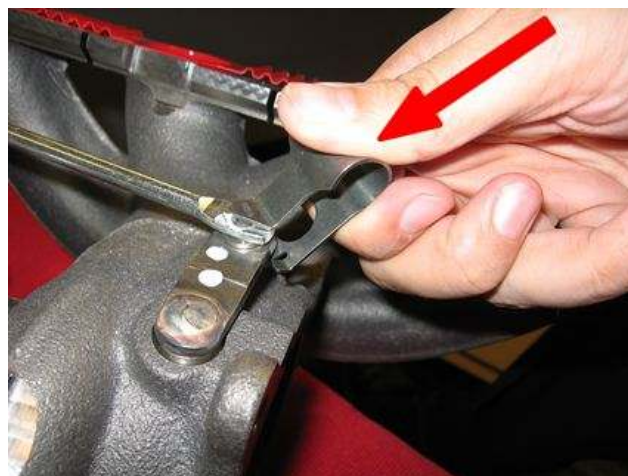
Figure 2. Fit the clip from the side.
