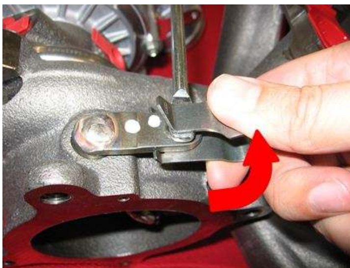
Figure 2. Turn the clip counter clockwise till the lugs slot in.
