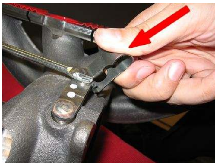
Figure 1. Fit the clip from the side.
