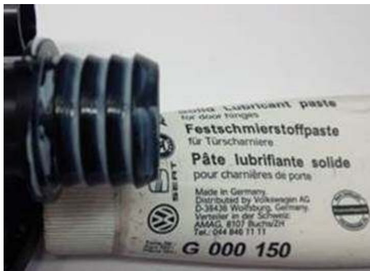
Figure 5. Grease film on outer surface of grommet.
