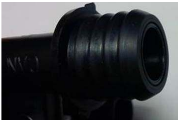
Figure 2. Align grommet and sensor outer edges.
