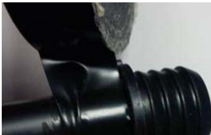
Figure 3. Wrapping vinyl tape behind the grommet.
