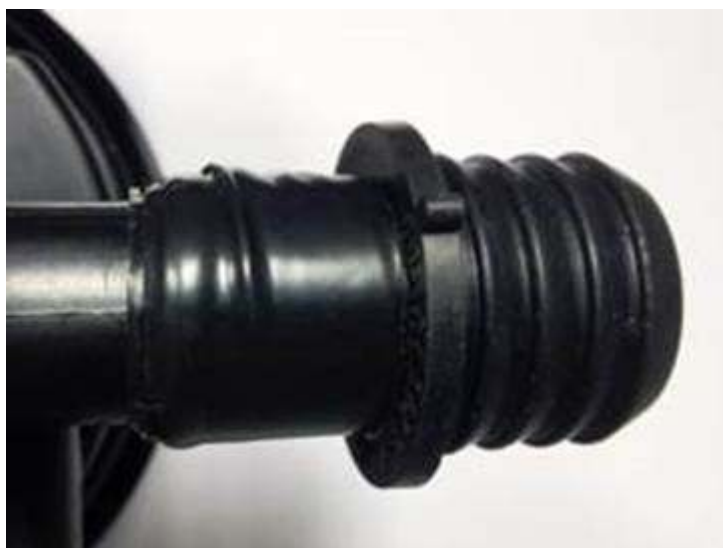
Figure 4. Vinyl layer supporting grommet.
