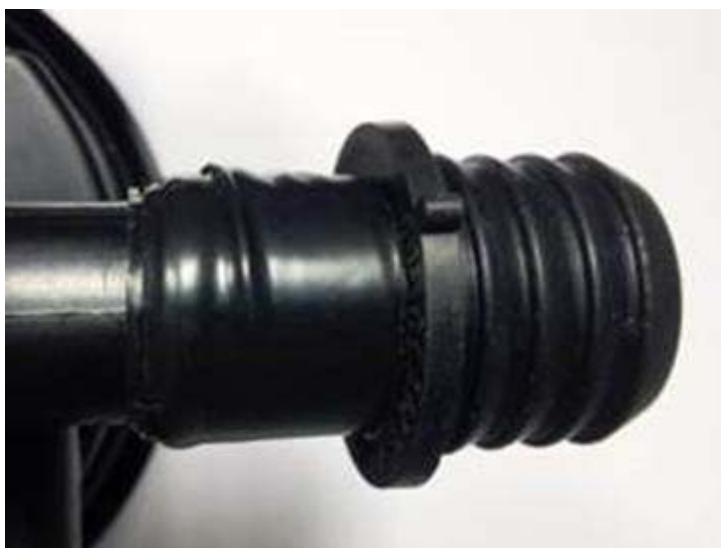
Figure 4. Vinyl layer supporting grommet.
