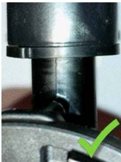
Figure 6. Correctly-installed sensor and grommet.
