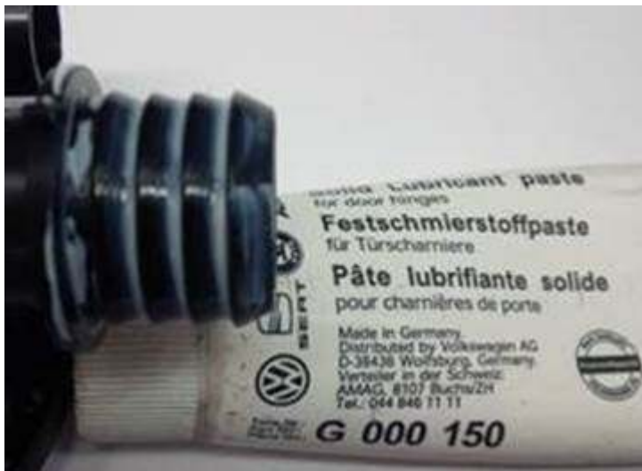
Figure 5. Grease film on outer surface of grommet.
