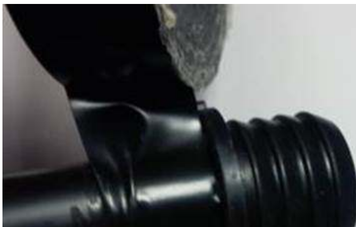
Figure 3. Wrapping vinyl tape behind the grommet.
