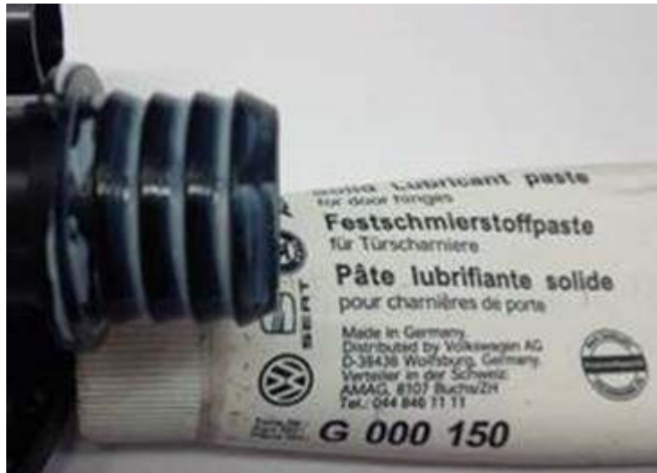
Figure 5. Grease film on outer surface of grommet.
