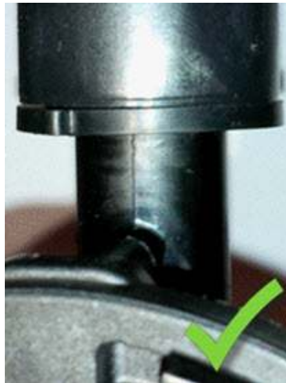
Figure 6. Correctly-installed sensor and grommet.
