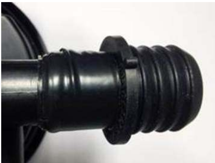
Figure 4. Vinyl layer supporting grommet.
