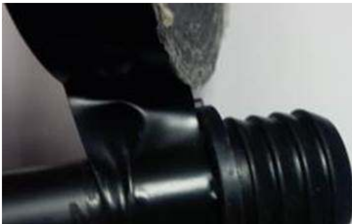
Figure 3. Wrapping vinyl tape behind the grommet.
