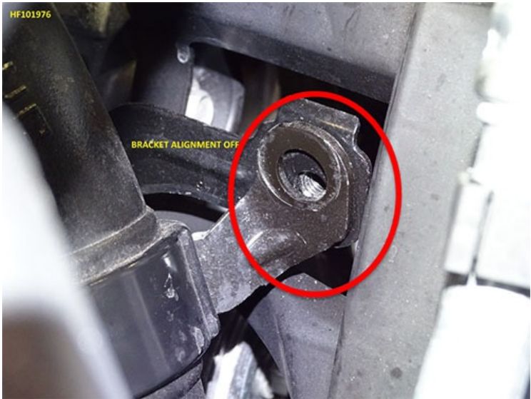
Mis-aligned charged air cooler pipe bracket and bolt hole after the charge air cooler outlet hose is connected properly to the throttle body.
