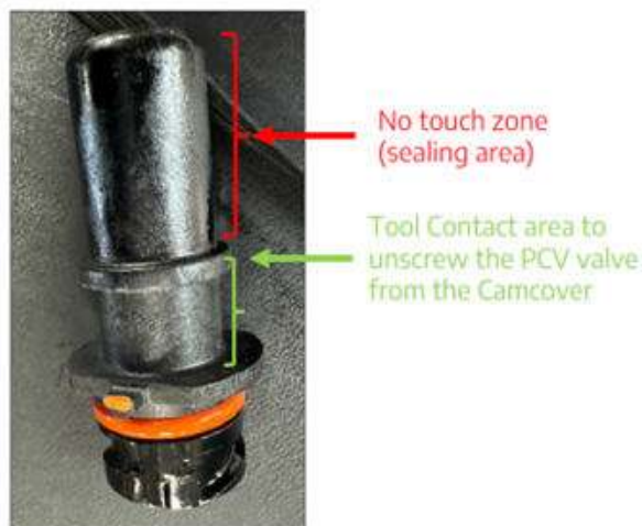
Fig. 1 PCV Valve During Removal
