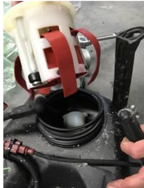
Figure 1. Filter element housing loose inside tank.
