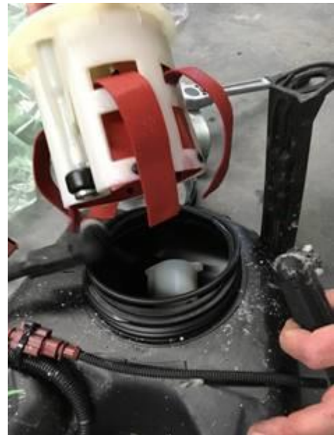
Figure 1. Filter element housing loose inside tank.
