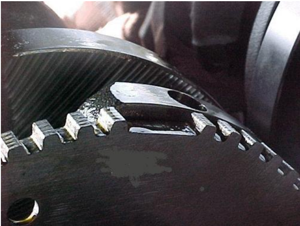
Crankshaft with bad reluctor wheel.
